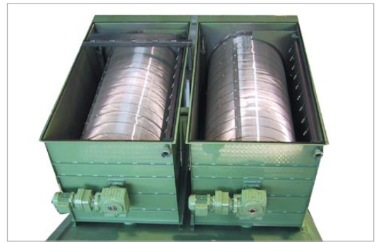
Drum sieve with stainless-steel sieves and nozzle carrier
