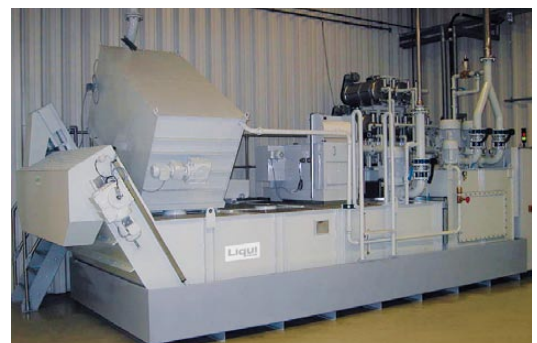
Drum sieve filter as coarse and pre-filter
